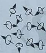
Fig. 4.6.1. Randomly oriented magnetic dipoles in a materials.
